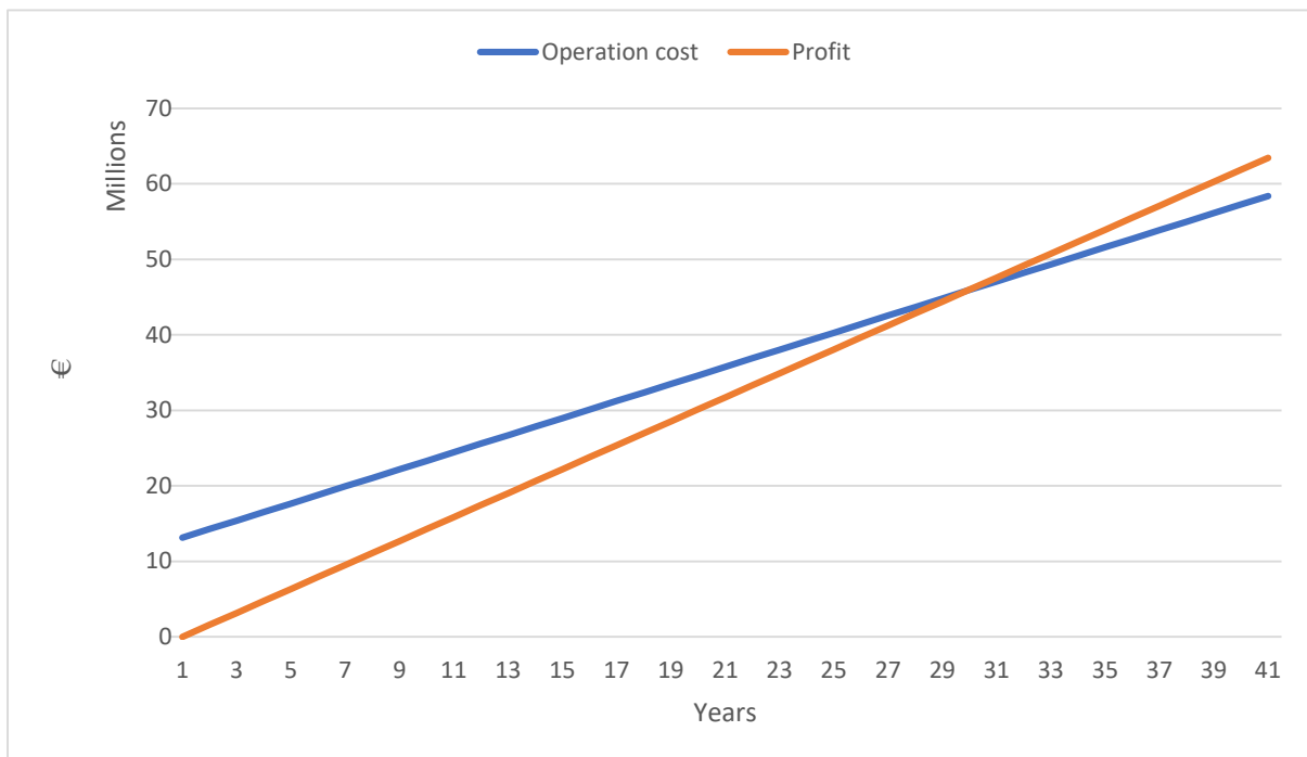
Figure 4.15: Profitability chart of 2 stages (Therminol) system
